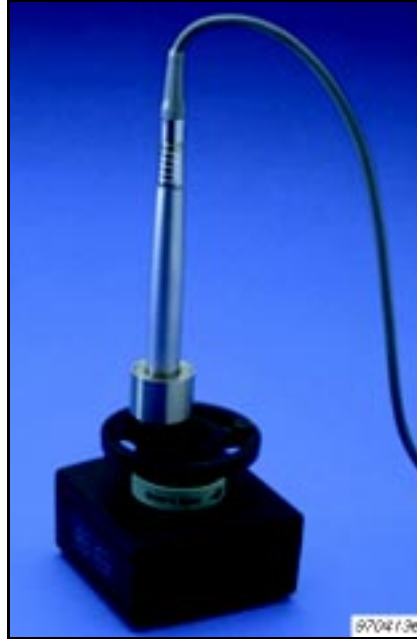
Fig. 8 Absolute sensitivity calibration at 1 kHz of Type 4195 using Sound Level Calibrator Type 4231 and Calibration Adaptor DP 0939
